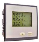
Three-phase network 340...450V (phase - phase) single-phase network 195...260V (phase - neutral) Connection with dedicated CT Programmable primary CT 5...8000A (41 ranges) True RMS value measurement
